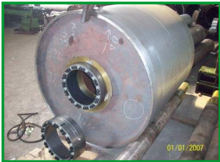
CONVEYOR PULLEY WITH RING FEEDER
